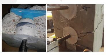
**GTI® GROUT-LOCK® Pocket Former**Prevents grout plug from pulling out; surrounding concrete fails in shear.
