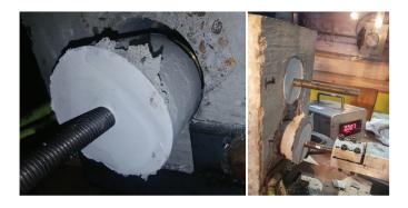
**Standard Grout Plug**Weak connection, poorly adhered to concrete. Grout pulls out as a conical plug; leaving anchorage unprotected.
