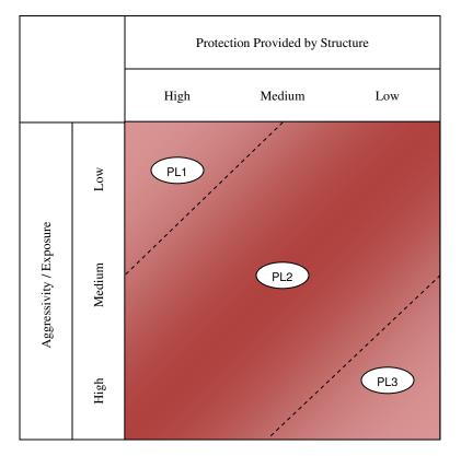
Following are examples for choosing tendon PL using Table 2 for a segmental concrete bridge.
