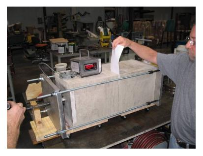
Figure 2: Testing of the GTI Gasket
